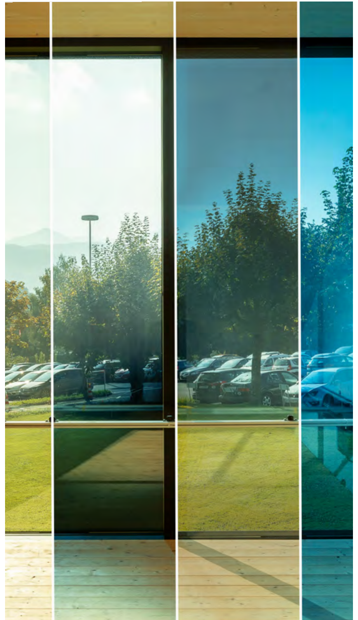
The window of the HSLU light measurement container shows four settings of the electrochromic glass (from left to right): untinted; continuous gradient from top, bright, to bottom, tinted; continuous gradient from top, tinted, to bottom, untinted; tinted. Photomontage: Licht@hslu
